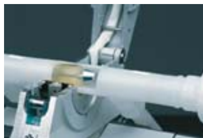
BCF® Bead and Crevice Free fusion technology - an internal bladder is positioned in the joint area for a bead and crevice free fusion. (picture Georg Fischer AG)
